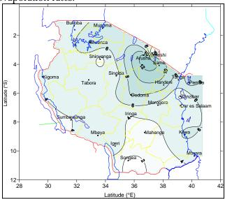
Figure 4: March 2009 Mean wind speed (km/hr)
